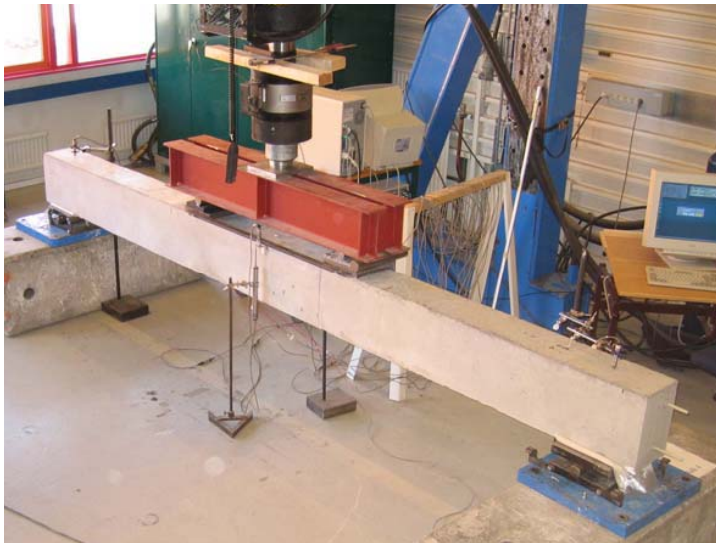
Figure 5-15. Picture taken on test setup during failure test.
