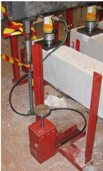
Figure 5-13. Left: The applied load is placed on the small piston. Right: The resulting load is created through a hydraulic cylinder.
