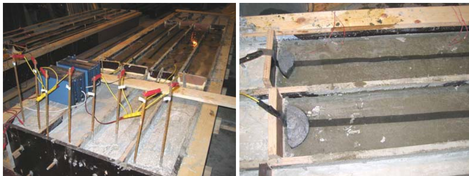
Figure 5-5. Left: Full view of initiation setup. Right: The anodic titan net placed in the water bath on top of concrete beam.
