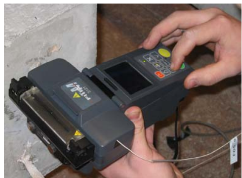
Figure 5-19. Left: Cross sectional view of optical fibre. Right: Splicing tool used to mend broken fibre.
