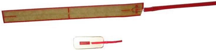
Figure 5-16. Top: Gauge used to measure strain on concrete with a length of 67 mm. Bottom: Gauge used to measure strain on glass fibre rod, steel reinforcing bars and CFRP plate. Scale 1:1.
