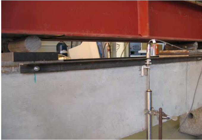
Figure 5-26. Curvature measurement setup using the 10 mm LVDT mounted on a steel profile reaching in between the loading points. Mid-point deflection is measured using a 100 mm LVDT.
