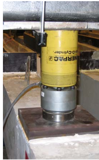
Figure 5-13. Left: The applied load is placed on the small piston. Right: The resulting load is created through a hydraulic cylinder.
